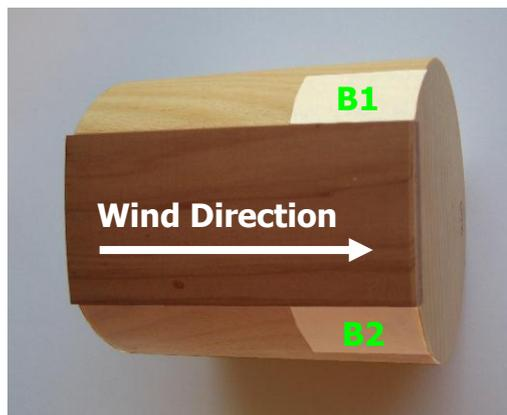
Practical use: If you switch from position 1 to position 2, the location of the bonded adhesive strips must be switched analogously to the directions. This can especially be the case if the block has risen due to the accrued humidity and is lying too high in relation to the labial edge (remove adhesive tape **A**, then bond new adhesive tape at **B1** and **B2**).
